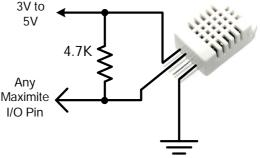
Where 'pin' is the I/O pin to which the sensor is connected. You can use any I/O pin but if the DHT22 is powered from 5V it must be 5V capable (ie, NOT a pin that supports analog input). The I/O pin will be automatically configured by MMBasic.
