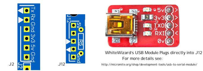
Generally, this is a 3 wire connection Tx, Rx & Gnd (if MuP is powered via J3) to an external USB to TTL adapter for communication with a PC but it may be convenient to use J2 or J12 as the entry point for the power supply as well. A classic example is when using a USB-Serial Cable similar to this unit available from DONTRONICS.COM
