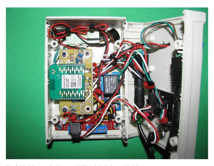
The finished Synapse Environmental RF Mesh Node Sensor Module.
