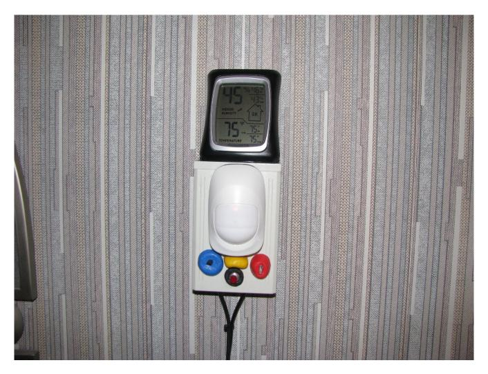
On the outside of the snap enclosure is the very reliable Visonic PIR pet immune motion sensor. Embedded in colorful silicon clay (Surgu) is the temperature sensor (blue), humidity sensor (yellow) light sensor (red) and the panic/ emergency push button (black). On top is my calibration reference module for my analog sensors.
