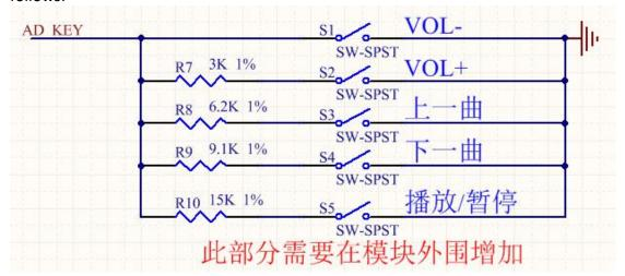
The R7-R10 four resistors are constructed with 1% precision resistors
