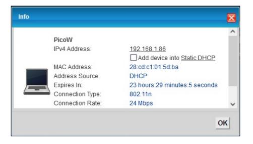
These IP numbers are generated by your router and automatically assigned to the devices. You can (if you want) assign IP numbers to the devices yourself. To do this you need to go into your routers software and make the alterations there. Generally a manual is supplied in which you can find how to do that.
