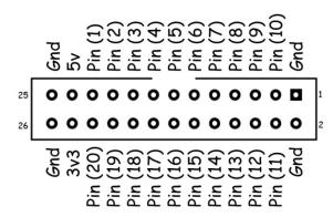
26 Pin Maximite GPIO Header (looking into Rear of Male Connector)
