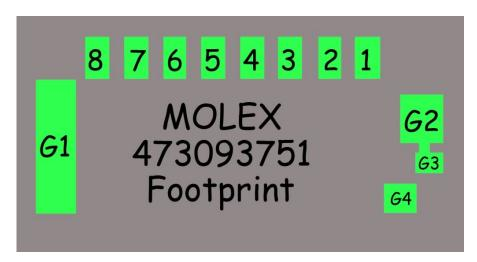
Next, manually align the uSD connector so that it fits perfectly to the outline on the PCB, (when viewed from above) then whilst holding it in place, carefully solder the G1 pad and check the alignment of the 8 electrical pins and the other pins. Reheat the joint and re-align if not satisfied. Solder the G2 pad on the other side and recheck before soldering the 8 data pins.
