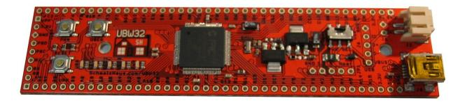
The UBW32 is a 4.4" x 1" (110mm x 25mm) PCB based on the Pic32 (MX795L) processor, designed by Brian Schmaltz and available for under \$40Aus from Dontronics.com and Sparkfun.com. Full details can be found at <a href="http://www.schmalzhaus.com/UBW32/">http://www.schmalzhaus.com/UBW32/</a>
