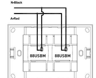
88USBM fitted to a wall plate
