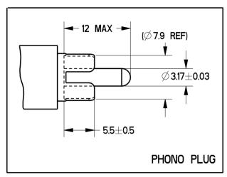
For dimensions which are not reflected in the drawing, refer to IEC 600169-24 (for F plug) and IEC 600169-2 (for IEC plug).
