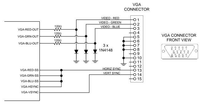
The I/O pins VGA-RED-CLK, VGA-GRN-CLK, VGA-BLU-CLK must be left unconnected.
