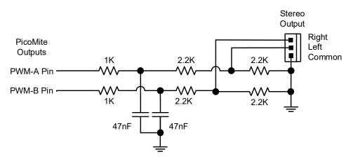
This circuit is suitable for general use; however more sophisticated designs can be used to improve the frequency response and reject more of the carrier frequency. This circuit is also suitable for generating a DC output signal using the PWM commands although, in that case, both 47 nF capacitors should be increased to 4.7  $\mu$ F to further suppress the PWM carrier frequency.
