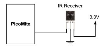
Vishay TSOP4838, Jaycar ZD1952 and Altronics Z1611A. Note that the I/O pins on the PicoMite are only 3.3V tolerant and so the receiver must be powered by a maximum of 3.3V.
