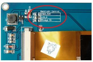
used to short the nearby pair of solder pads marked "1963-PWM". The PicoMite can then control the brightness via the SSD1963 controller using the BACKLIGHT command.
