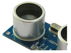
This device can be found on eBay for about \$4 and it will measure the distance to a target from 3cm to 3m. It works by sending an ultrasonic sound pulse and measuring the time it takes for the echo to be returned.
