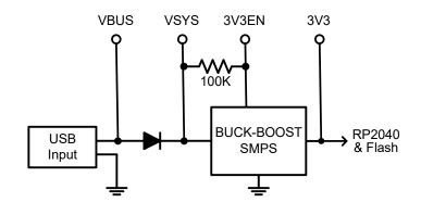
For embedded controller applications generally an external power source (other than USB) is required and this can be connected to VSYS via a Schottky diode. This will allow the PicoMite to be powered by whichever supply is producing the highest voltage (USB or VSYS). The diodes will prevent feedback into the lower voltage supply.
